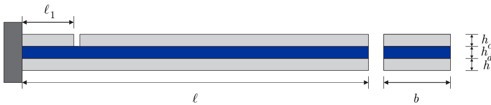
Figure 6.75 Cantilever beam with segmented constraining layer
