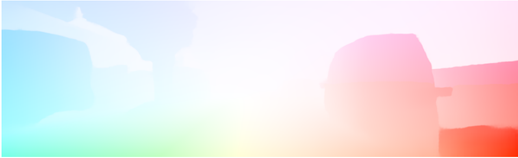
(b) Optical flow visualisation with a circular colour palette, where each colour corresponds to a specific flow direction.
