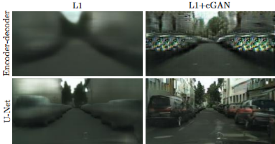
Figure 3.10: Incorporating skip connections within an encoder-decoder architecture, forming a U-Net inspired architecture, significantly enhances the overall quality of the outcomes, (from [51]).
