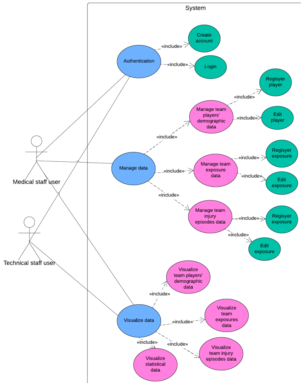
Figure 4.1: Use case diagram of the mobile application
