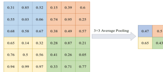
Figure 3.10: Average pool operation with kernel 3 \times 3 from [14].
