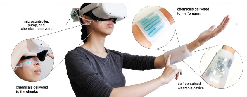
Figure 2.23: Process of providing chemicals to simulate different sensations [27].
