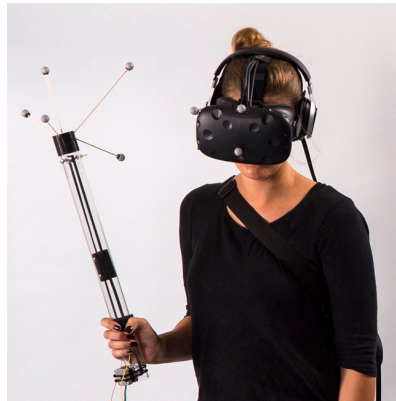
Figure 2.18: Shifty graspable haptic device [39].
