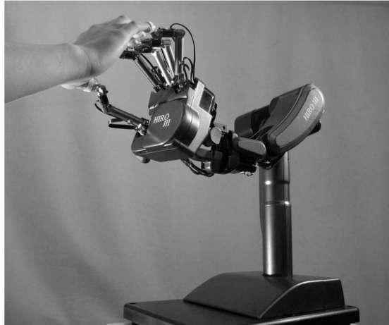
Figure 2.24: Hiro-III haptic device [13].
