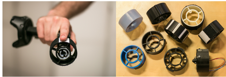
Figure 2.14: Modularity of the Haptic Revolver [37].
