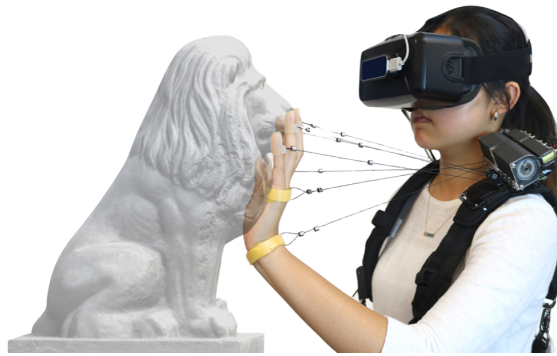
Figure 2.11: Wireality simulating a complex shape [14].
