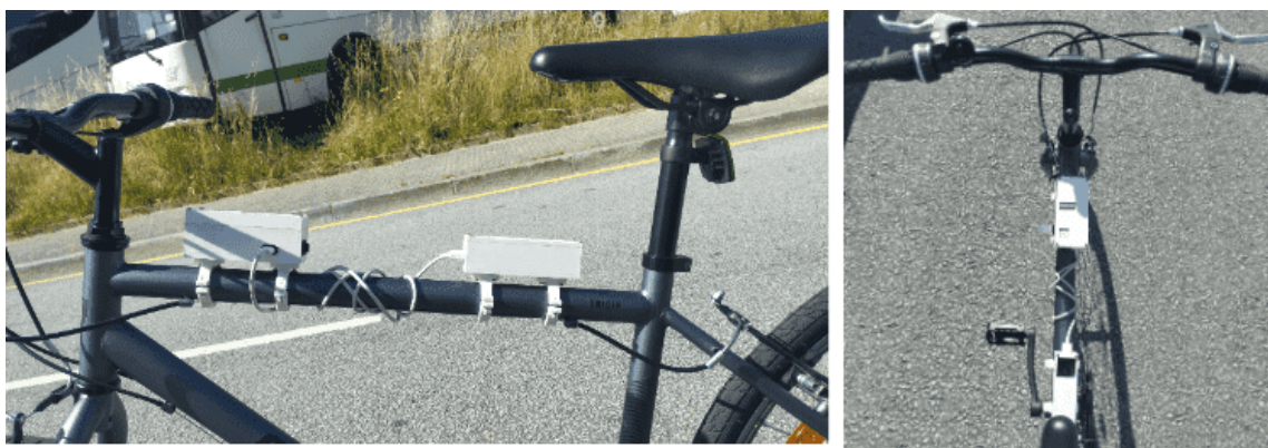
Figure 4.6: Real life final assemble of the MobiAlert unit attached to a bicycle.
