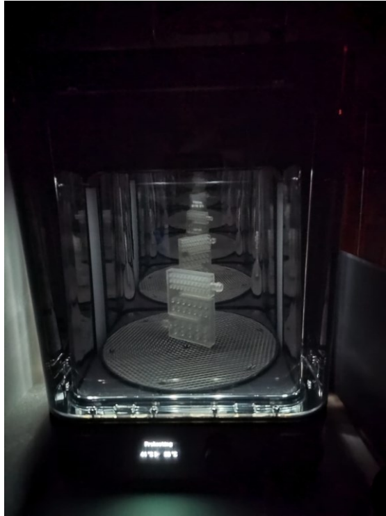
Figure Appendix J. 5: Image of the printed piece while the cure device is pre-heating.
