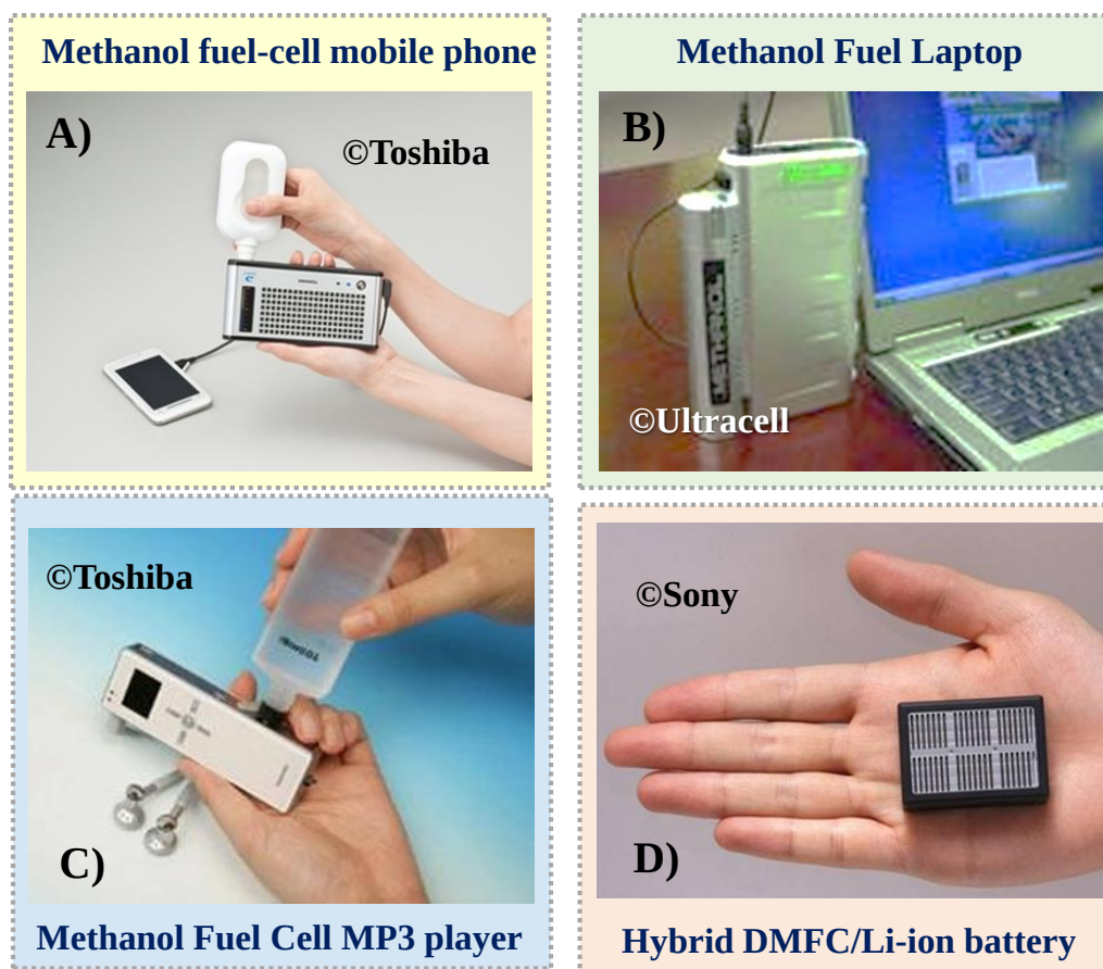
Figure 2.21 – Direct Methanol Fuel Cell portable prototypes, including a methanol fuel cell mobile phone launched by ©Toshiba (A), a portable laptop powered by a methanol fuel cell launched by ©Ultracell (B), a methanol fuel cell MP3 player launched by ©Toshiba (C), and a hybrid fuel cell system integrating a DMFC and a Li-ion battery launched by ©Sony (D).
