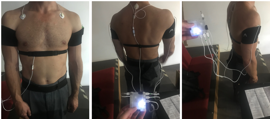
Figure 7.1: The sensors are attached to specific points on the body, which are likely chosen for their relevance to the type of data being collected. For example, electrodes on the chest can be used for an electrocardiogram (ECG) to measure heart activity, while those on the back and arms might be for electromyography (EMG) to record muscle activity.
