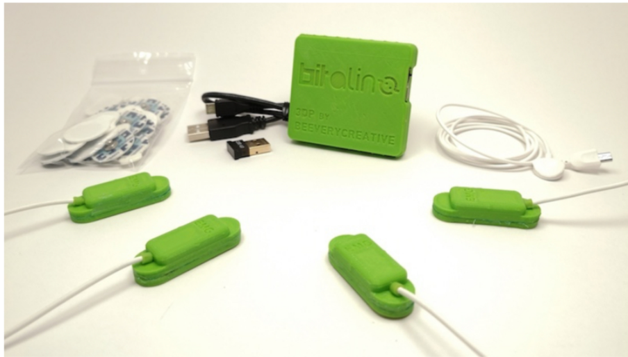
Figure 5.1: The BITalino platform offers various bundles to cater to different needs, ranging from basic to more advanced setups. These bundles typically include a variety of modular sensors, the main BITalino board, and sometimes additional accessories like cables, electrodes, and power supplies. The idea is to provide a comprehensive package that allows users to get started with physiological data acquisition right out of the box.
