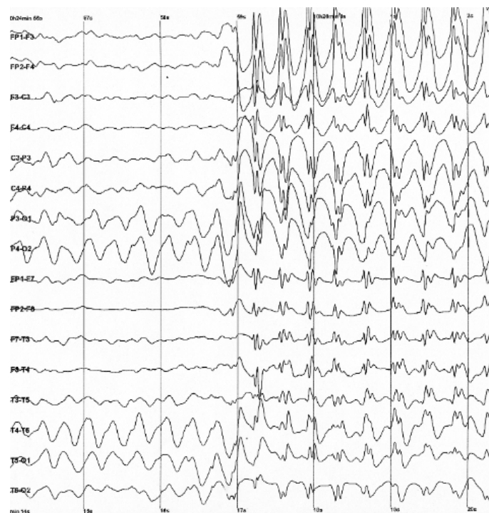
Figure 4.9: The image depicts an Electroencephalogram (EEG) signal. EEG is a method used to record the electrical activity of the brain. The plot has multiple channels, each labeled with specific acronyms. These labels typically denote the specific electrode placement on the scalp, corresponding to different brain regions. For instance, "FP" usually stands for frontal-polar, "F" for frontal, "C" for central, "P" for parietal, "O" for occipital, and so on. The waveform for each channel represents the brain's electrical activity at that specific location. EEG signals typically consist of rhythmic waveforms that can vary in frequency and amplitude. The waves might indicate different stages of wakefulness or sleep or different cognitive processes. Some sections of the EEG display appear to be more erratic or of larger amplitude than the typical brain waves. These could be artifacts, which are unwanted or non-brain signal interferences. Artifacts can be caused by various sources like eye blinks, muscle movements, or external electrical interferences.
