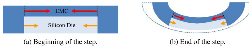
Figure 2.28: Illustrative depiction of the CTE mismatch impact on warpage after the curing process, above T_g , of the epoxy mold compound.
