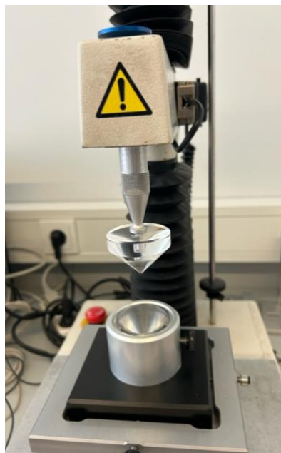
Figura 17. Texturómetro Stable Micro Systems TA-XT2i e sonda TTC Spreadability Rig (HDP/SR) .
