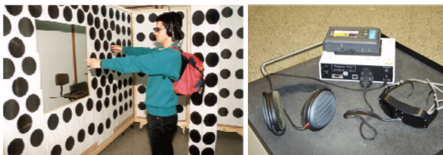
Fig. 2.2L "Picture of a user performing a training task, moving around fake walls and columns and trying to identify the whole environment; The final prototype was composed by a 3d distance sensor (glasses), the control and sound generation hardware and a pair of headphones." (Torres Gil et al., 2010)
