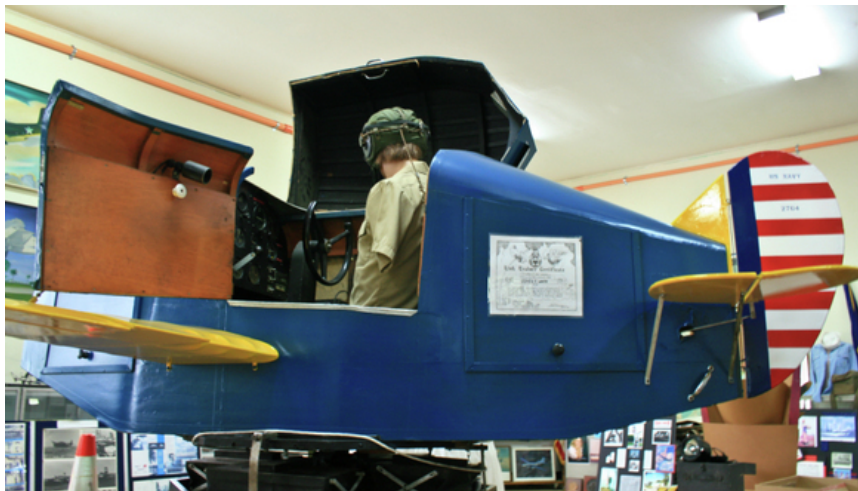
Fig 2.1C "Link Trainer Flight Simulator on Exhibit © NAS Fort Lauderdale Museum" (McElhiney, n.d.).
