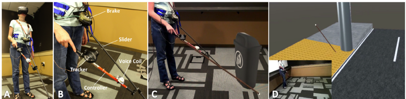
Fig. 2.2J “(A) A blind user wearing the gear for our VR evaluation, including a VR headset and Canetroller, our haptic VR controller. (B) The mechanical elements of Canetroller. (C) Overlays of the virtual scene atop the real scene show how the virtual cane extends past the tip of the Canetroller device and can interact with the virtual trash bin. (D) The use of Canetroller to navigate a virtual street crossing: the inset shows the physical environment, while the rendered image shows the corresponding virtual scene. Note that users did not have any visual feedback when using our VR system. The renderings are shown here for clarity.” (Zhao et al., 2018)
