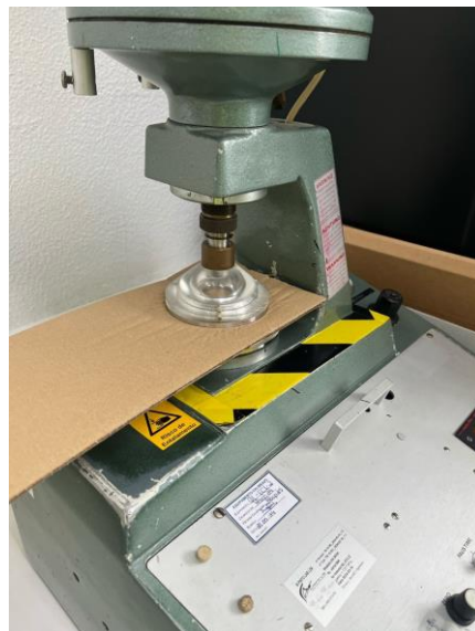
Figure 3.27 – Mullen test process
