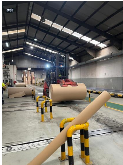
Figure 3.5 - Supply of reels by forklift
