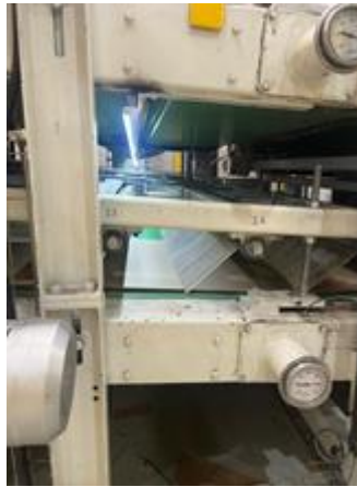
Figure 3.18 - Stabilization mechanism after cutting
