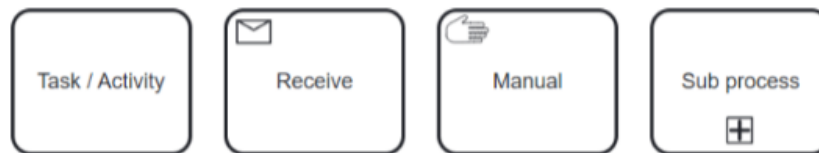
Figure 2.4: Types of actions in the BPMN Source: BPMN.IO (2022)
