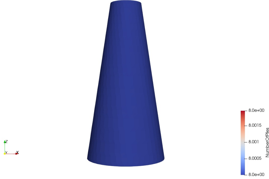
Figure 3.25: Cone model ply count distribution
