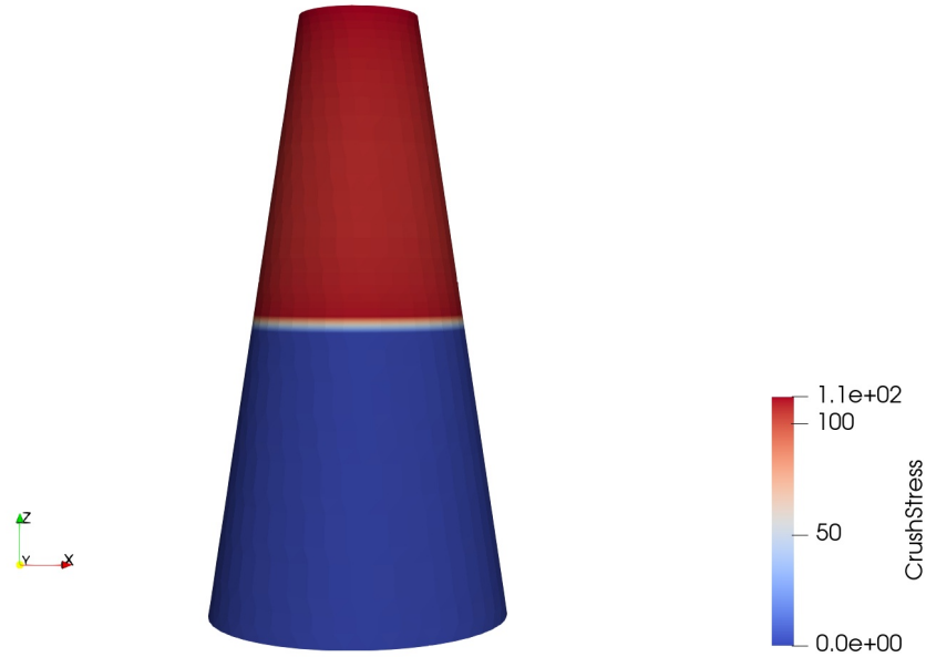
Figure 3.35: 3D crush stress field for a dynamic, 8-ply carbon fibre cone simulation
