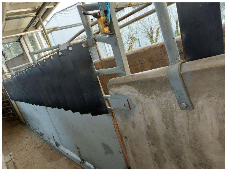
Figure C1. Rubber structures on the sides of the race leading animals to the stunning point, at the PEC Nordeste Slaughterhouse.
