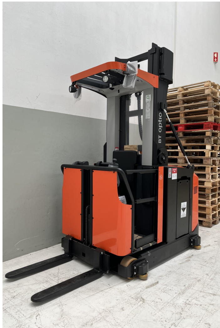
Figure F.1: Picture of the order picking machine
