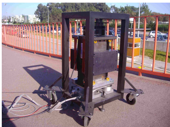
Figure 11. a) View of the actuator; b) Load cells responsible to measure interaction forces
