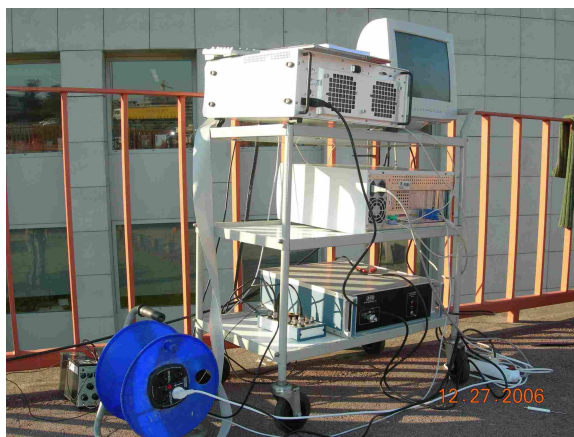
Figure 12. a) Accelerometer used to measure the system response; b) Controller and host computer
