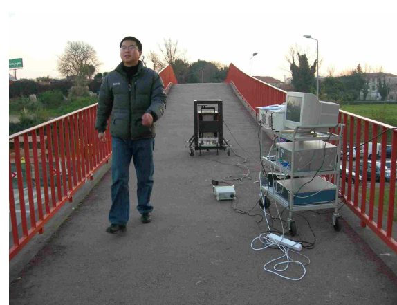
Figure 13. a) Pedestrian skipping near the actuator; b) Pedestrian walking along the footbridge
