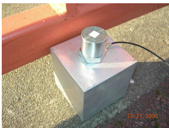
Figure 12. a) Accelerometer used to measure the system response; b) Controller and host computer
