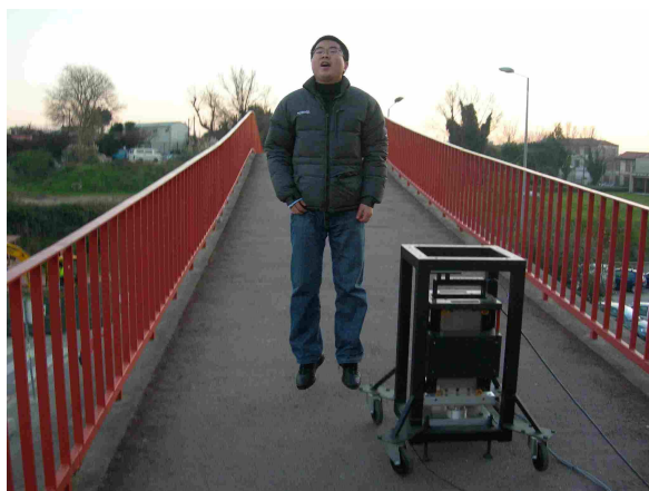
Figure 13. a) Pedestrian skipping near the actuator; b) Pedestrian walking along the footbridge
