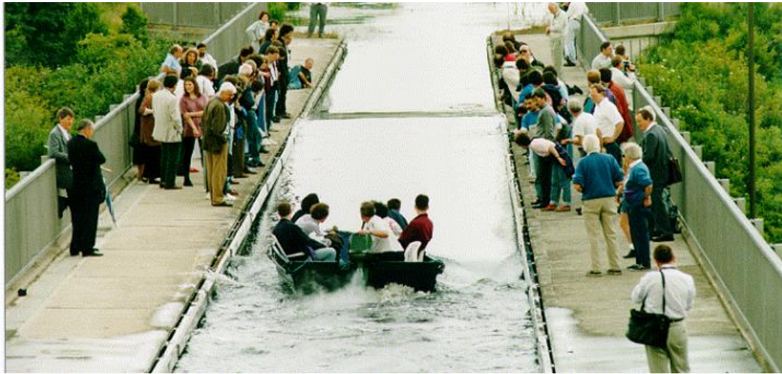
Figure 1.4 - A surface soliton is shown propagating in a narrow water channel, which was recreated in an experiment similar to that of Sir Scott Russell in 1834. Note how the solitary wave propagates ahead of the boat as it decelerates and comes to a full stop. See more at http://ramanujan25449.blogspot.com/2017/05/solitones.html .
