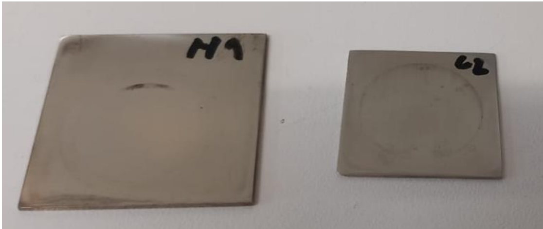
Figure 16: Visual examination of the charging side of the samples after permeation.
