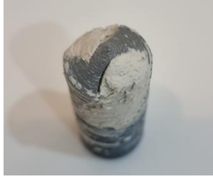
Figure 3. BKS with the material inside after total collection and removal. The MRT result was 25 N/cm.
