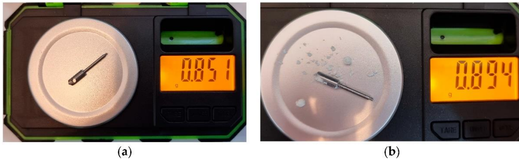
Figure 5. (a) BKS original weight; (b) BKS and bone weight measurement after total bone removal. The total bone weight is obtained by subtracting the weight of the BKS with bone from the original weight (43 mg).
