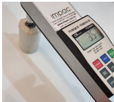
Figure 2. The Lutron Digital Torque Wrench (TQ8801) displays 35 N/cm (MIT).
