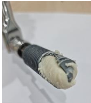
Figure 3. BKS 3D printed filled with aluminum phyllosilicates (clay) after insertion and removal of the BKS into the material tested [8].
