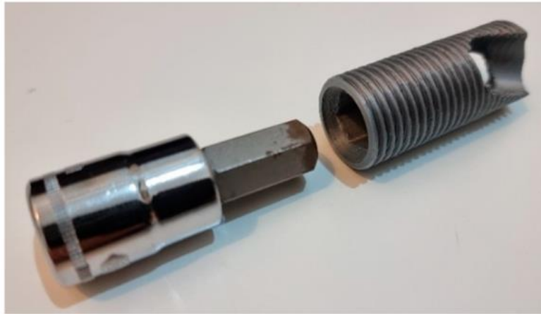
Figure 4. Testing connections in the BKS 3D printed in composite (Nylon).
