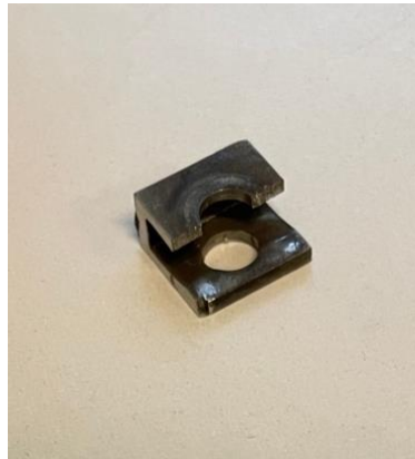
Figure 4-17 – Gripper after critical failure.
