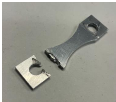
Figure 4-32 – Specimen 3 after the fracture.
