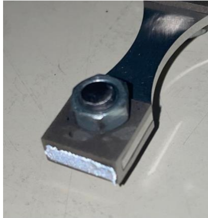
Figure 3-6 – Picture of gripper with reflective paper.
