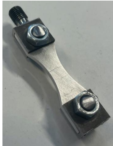
Figure 4-29 – Specimen 1 after the cracking.
