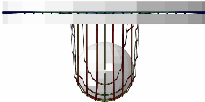
Figure 51 Numerical model results on the ball burst test conducted on meshes.
