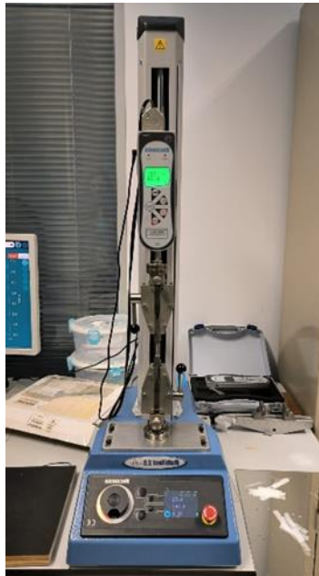
Figure 17 Uniaxial tensile test machine used to perform uniaxial tensile tests.
