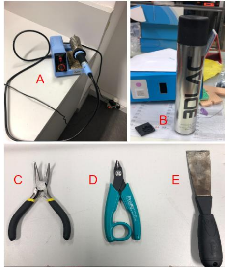
Figure 34 - A - soldering equipment; B - Hair spray; C - Plier; D - Cutting Clamp; E - Spatula.
