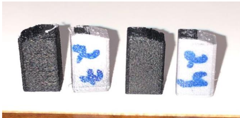
Figure 79 - Good surface quality and very good surface quality respectively, samples 27 and 24 respectively.
