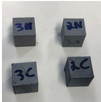
Figure 39 - Samples chosen for the shape analysis: 2N - Version 2 natural filament; 3N - Version 3 natural filament; 2C - Version 2 CB /TPU filament; 3C - Version 3 CB/TPU filament.
