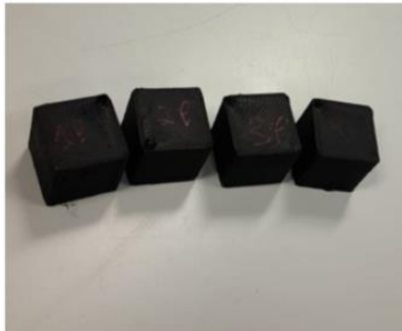
Figure 62 - Calibration cubes version 1.2 in CB/TPU.
