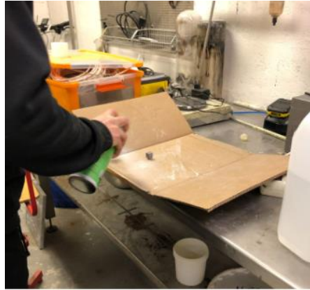
Figure 40 - Spraying of the samples to be scanned.
