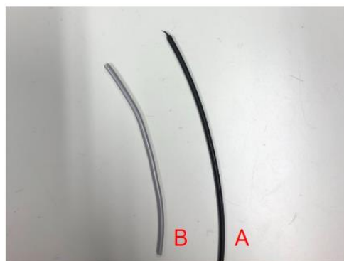
Figure 24 - Segments used for FTIR analysis: A - natural TPU; B – CB/TPU.
