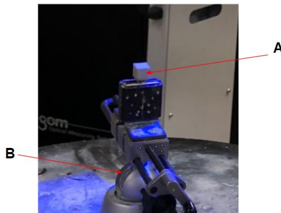
Figure 41 - Samples positioning 3D scanning: A - Bottom layer; B - Support.
