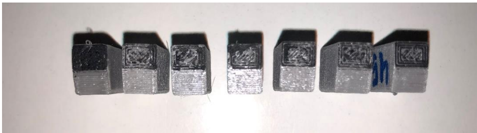
Figure 96 - From left to right: Fracture region of samples P_bp_1, 23, 24, 29, 30, 40, and 45.
