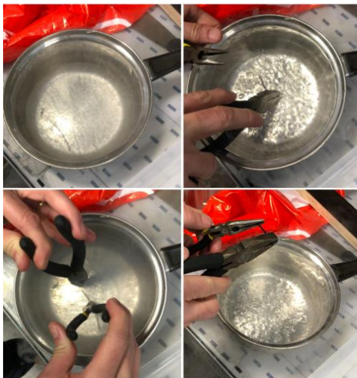
Figure 48 - Cryogenic fracture of the segments.
