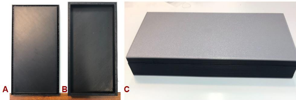
Figure 98 - EMI shielding case: A – Cover; B – Base; C - Assembly.
