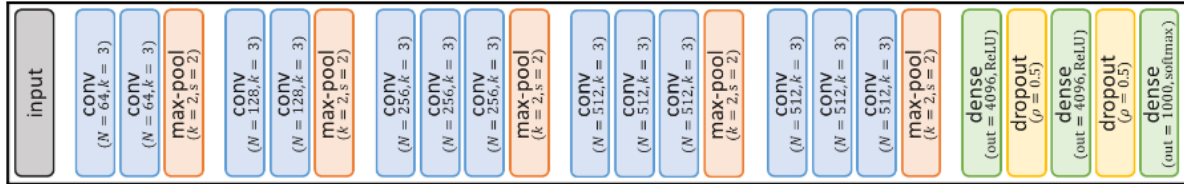
Figure 2.7: VGG-16 architecture. Image source: [50]
