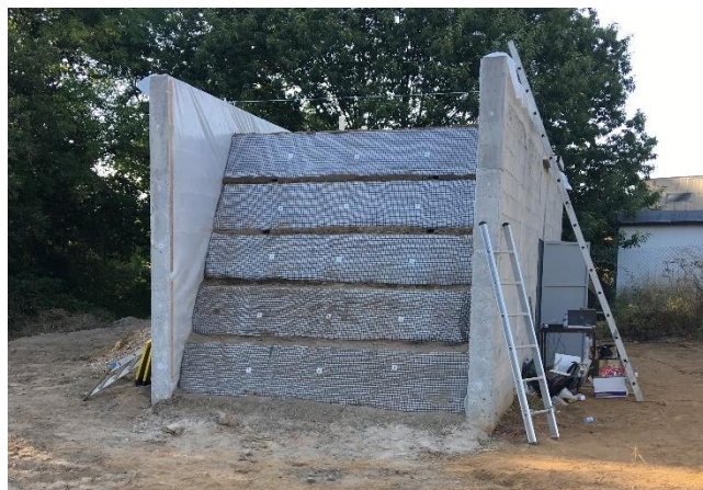
Figure 6. Full-scale geosynthetic-reinforced structure built with recycled C&D waste (Ferreira et al. 2022; Vieira et al. 2023).
