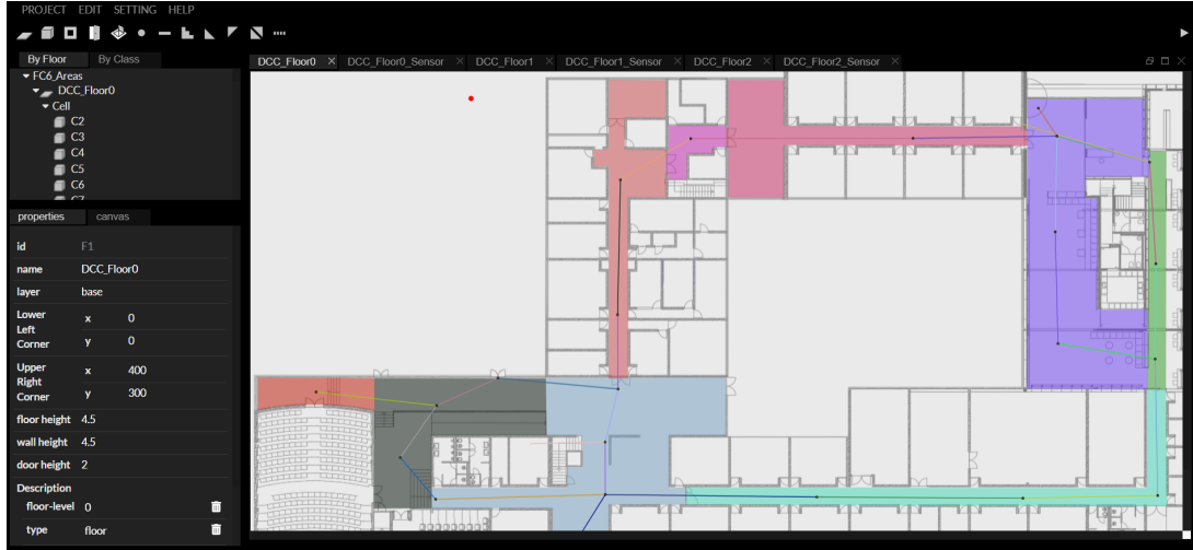
Figure 4.3: Example of IndoorGML Navigation Paths
