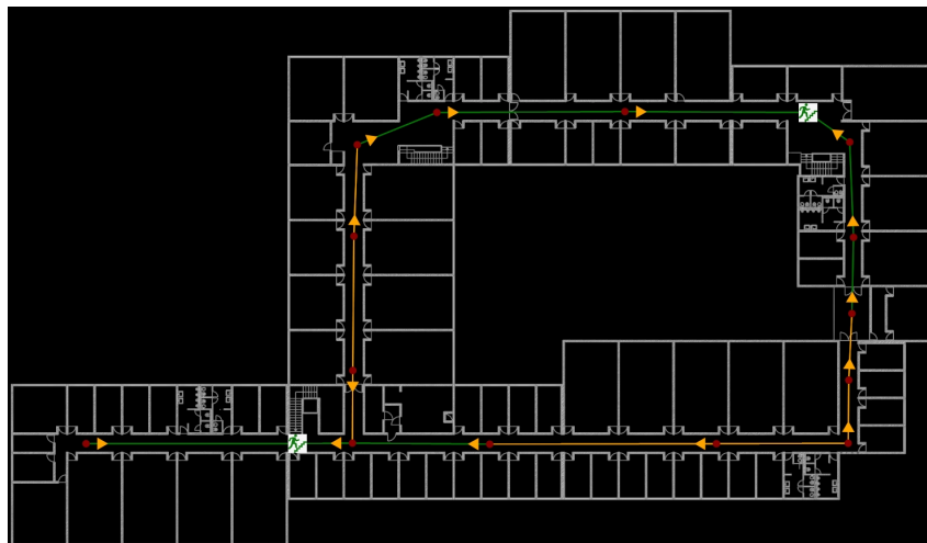
Figure 6.24: Test Case 4: DCC Floor 1 Exit Paths
