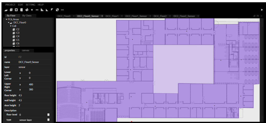
Figure 4.4: Example of sensor layer in IndoorGML
