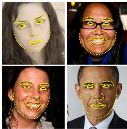
Figure 2.4: Example of landmarks detected in some faces [28]
