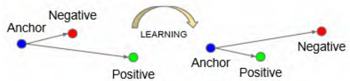
Figure 2.5: Visualization of the Triplet Loss process [40]
