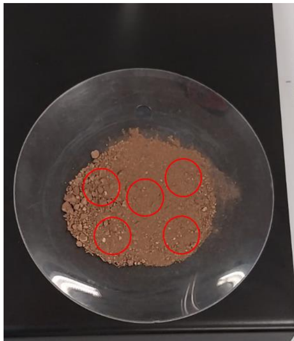
Figure 13: Soil spread in the watch glass and represented disposition of the measurements taken.
