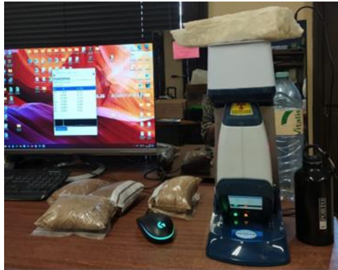
Figure 11: Bruker S1 Titan X-ray Fluorescence Analyzer used for the geochemical analysis of the samples.
