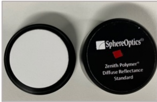
FIGURE 5.1: 99% Lambertian Source: Zenith Lite diffuse targets
