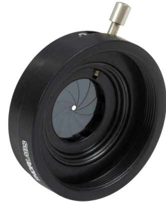
FIGURE 3.9: Lever-Actuated Iris. Source:[35]
