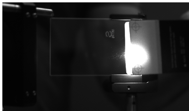
FIGURE 5.5: Image captured by the camera during the alignment of the mirror, illustrating the utility of the VIS/NIR Detector Card and the camera in visualising the beam's location.
