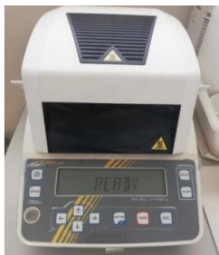
Figure 3. Infrared balance (KERN DBS, Baligen, German).
