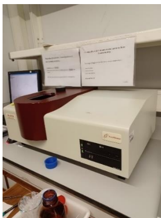
Figure 23. Particle size analyser, Brookhaven Instruments.
