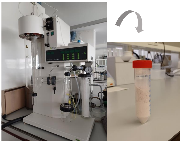
Figure 22. BÜCHI Mini Spray Dryer (left image); final spray dried powder (right image).
