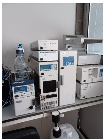
Figure 7. HPLC-DAD-FLD system (Jasco Corporation).
