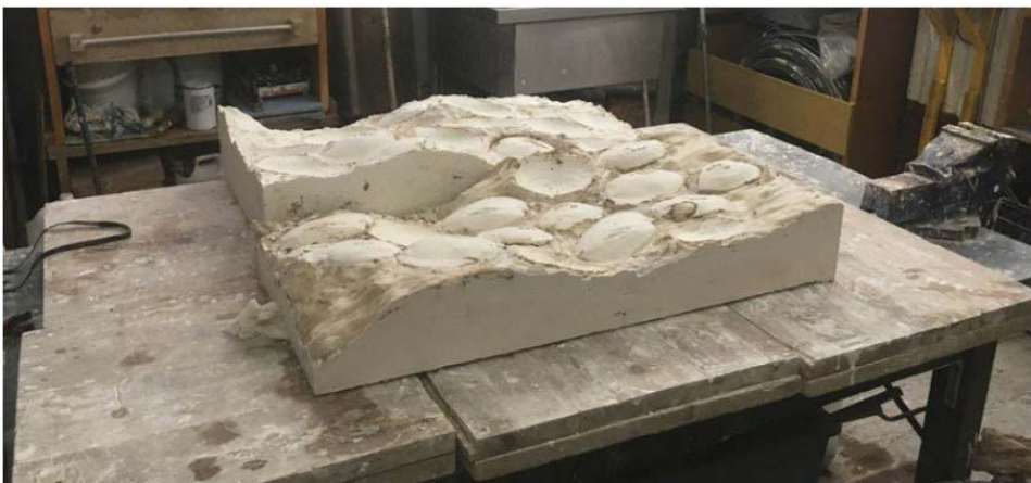
Fig. 26.: Process image of plaster and silica mould, 44,5 x 87 x 4- 13 cm.
