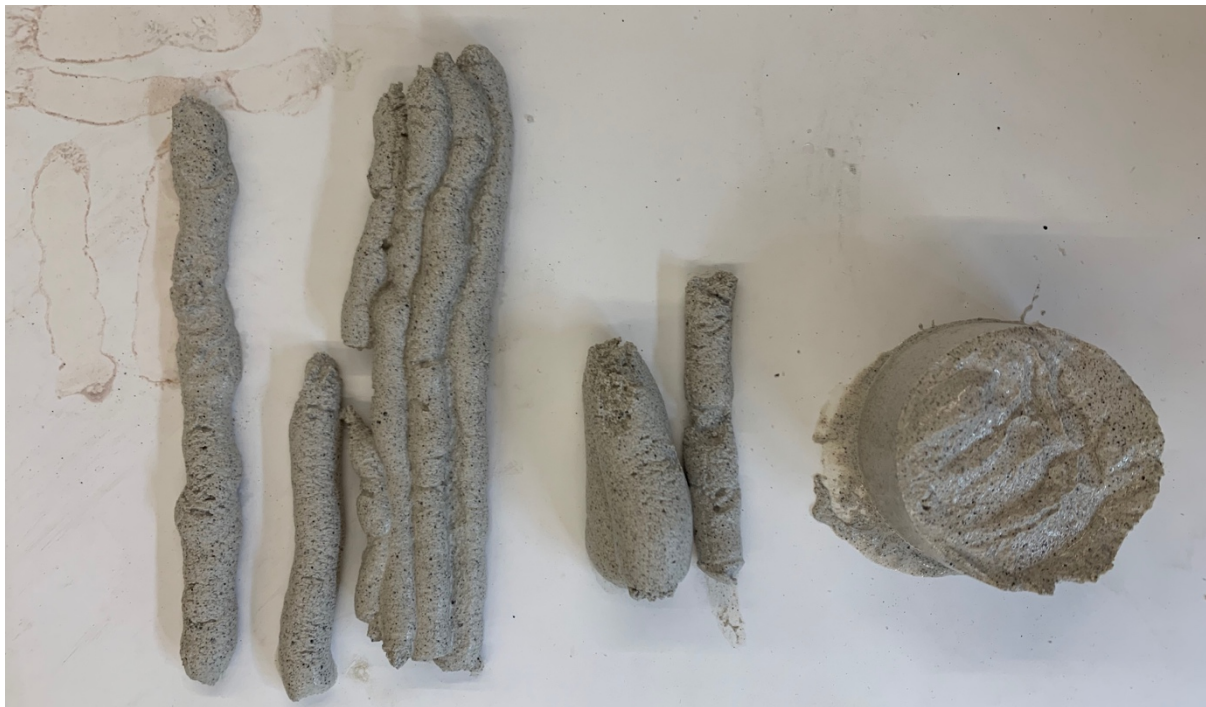
Figure 66. Test 9 - on the left extrudability tests and on the right slump test
