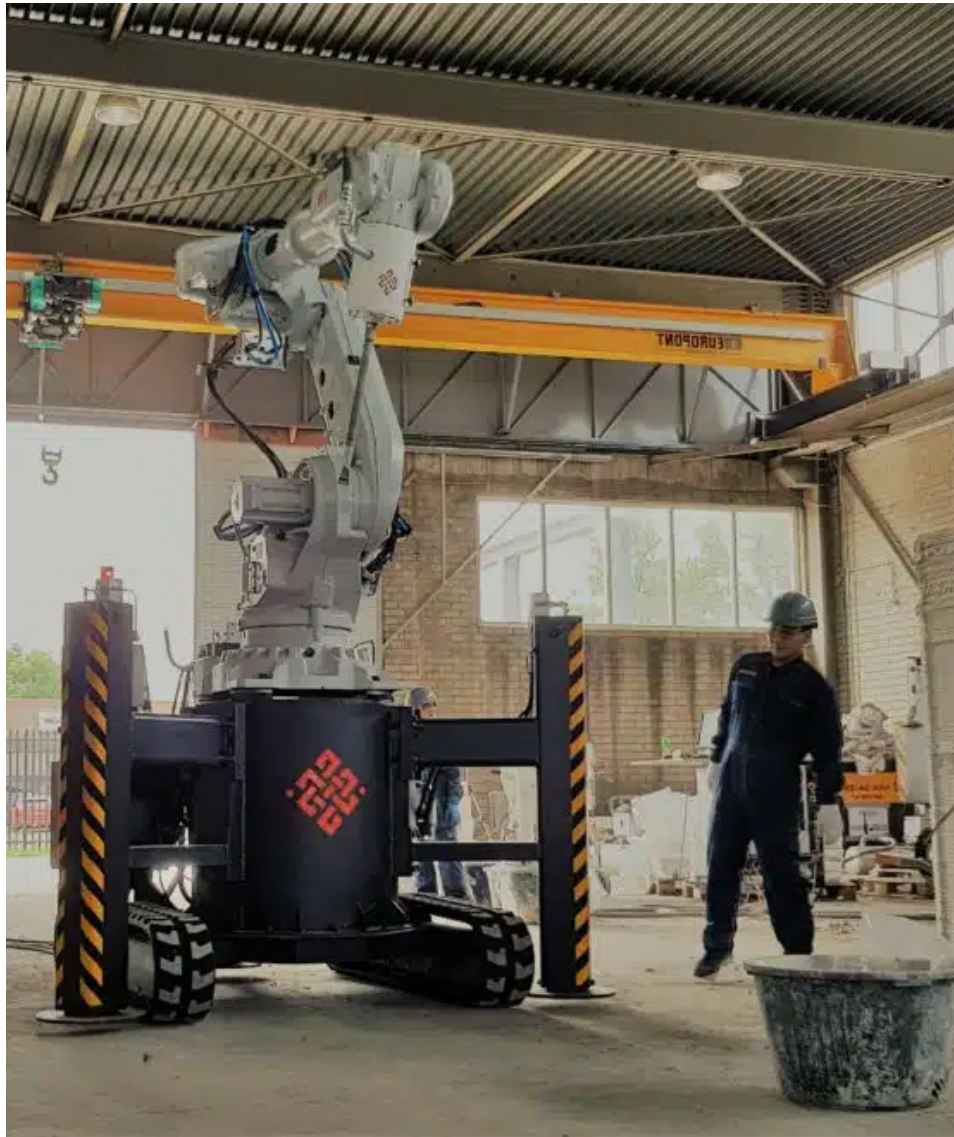
Figure 16. CyBe RC (robot crawler)/3D Concrete Printers | CyBe Construction, n.d.)
