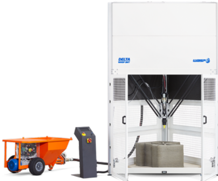
Figure 9. Delta Wasp 3MT (Concrete 3D Printer Delta WASP 3MT CONCRETE, n.d.)
