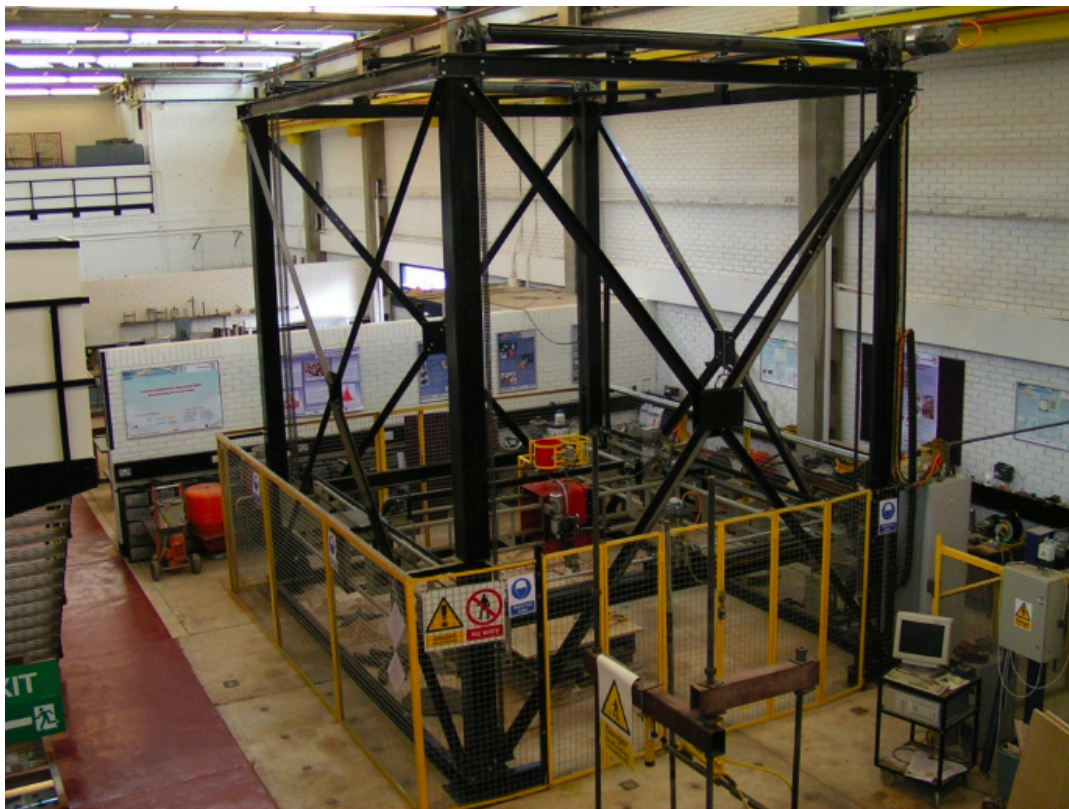
Figure 12. The printing frame for concrete printing (Lim et al., n.d.)
