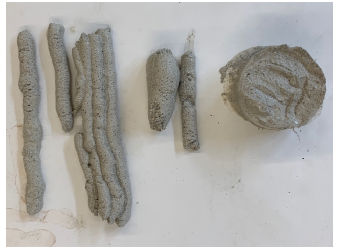
Figure 81. Extrudability and buildability test
