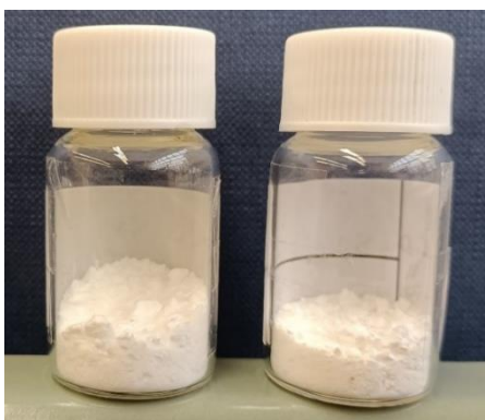
Figure 3.1 – Mesoporous silica materials prepared: SBA-15 (on the left) and APTES-SBA-15 (on the right).
