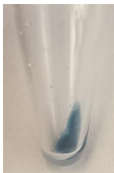
Figure 3.12 – Image of the \text{H}_3\text{PMo}_{12}\text{@APTES-SBA} composite after catalytic reaction.
