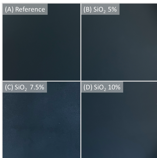
FIGURE 4.23: Samples with (A) Exterior grade film and decorative paper with (B) 5 wt%, (C) 7.5 wt% and (D) 10 wt% SiO 2 nanoparticles concentration.
