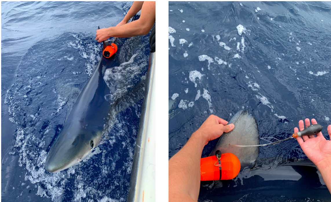
Figure 2. Double tagging. DOME (Dissolved Oxygen Measuring) archival tag with oxygen, temperature and accelerometer sensors using a zip-tie with an explosive timed release (48h) and a PSAT tag attached to the dorsal fin of a 272cm TL female blue shark ( P. glauca ) in Azores archipelago. Photo: CIBIO/Luana Coelho.
