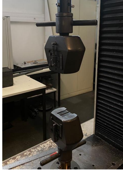
Figure 22 - Photograph of the equipment used in the tensile tests
