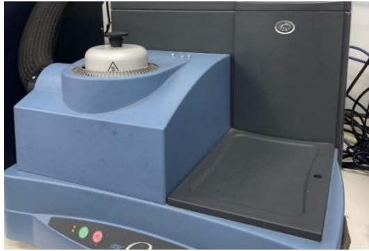
Figure 18 - Photograph of the equipment used in the DSC tests - Model Q20 from TA Instruments ®
