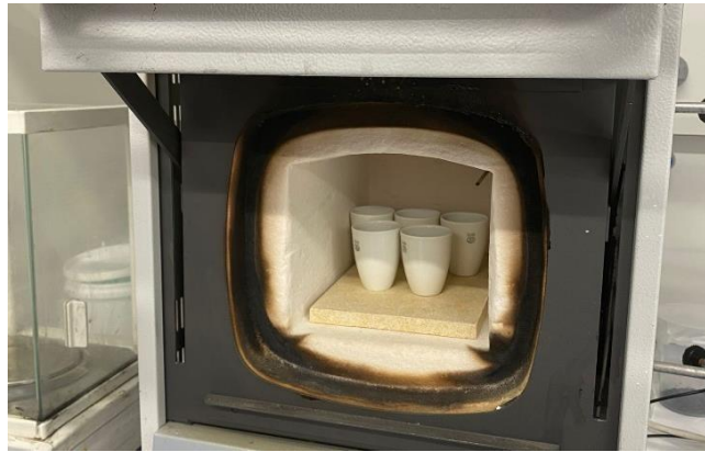
Figure 17 - Muffle furnace used in the fiber content and void volume test.
