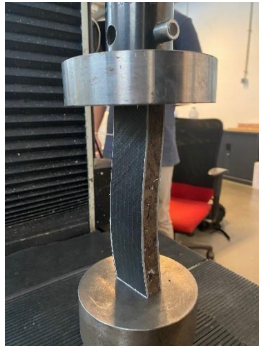
Figure 21 - Photograph of the equipment and sample used in the compression tests.
