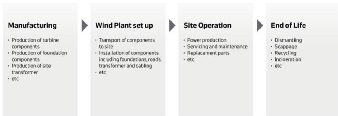
Figure 11 – Life Cycle Stages of a wind turbine. [69]
