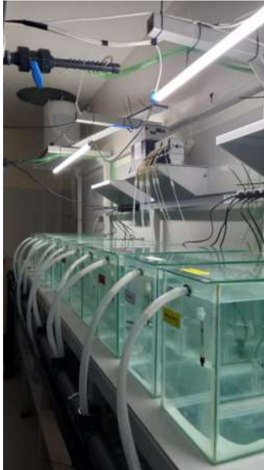
Figure 5- Long-term toxicity bioassay's setup.
