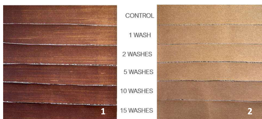
Figure 49: (1) Samples of the material designed with pine bark waste that were tested for colour fastness to washing; (2) Samples of the material designed with pine sawdust waste that were tested for colour fastness to washing.
