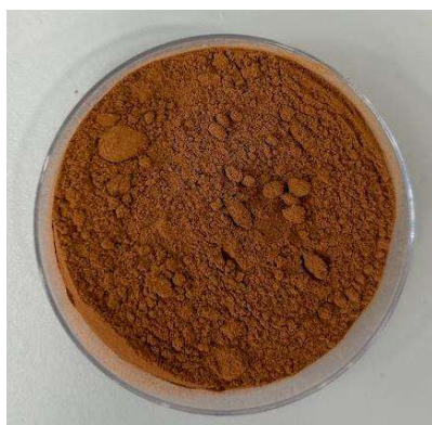
Figure 27: Pine bark particle size after the ball milling process
