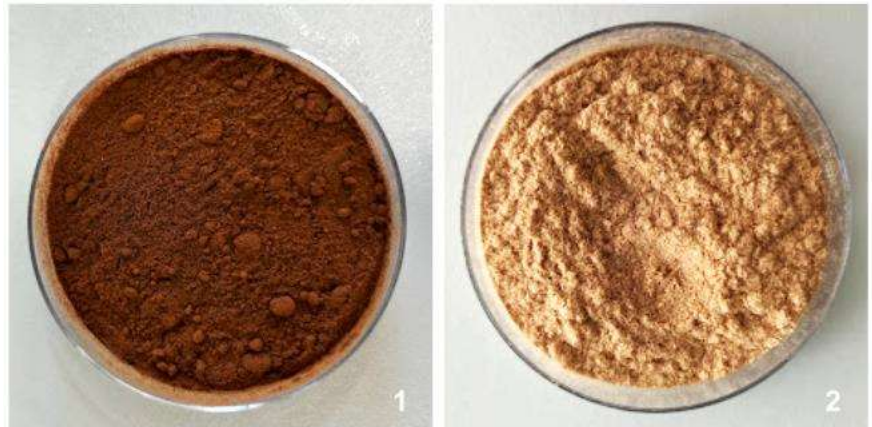
Figure 26: (1) Pine bark and (2) sawdust particle size after the manual sift process.
