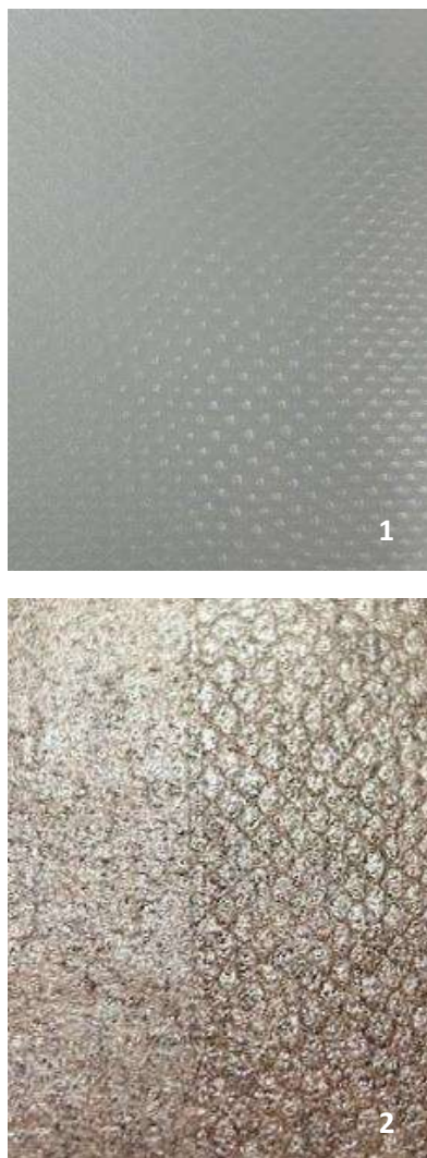
Figure 7: Example of an embossing. (1) The pattern used to create the texture on the surface; (2) the coated surface after the embossing process. It is visible where it was applied and where it wasn't.
