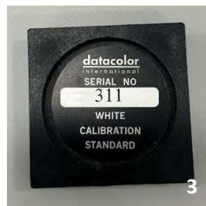
Figure 54: Patterns to calibrate the machine Datacolor® Spectraflash® SF450®. (1) and (2) different views of the black standard for the calibration; (3) and (4) different views of the white standard for the calibration
