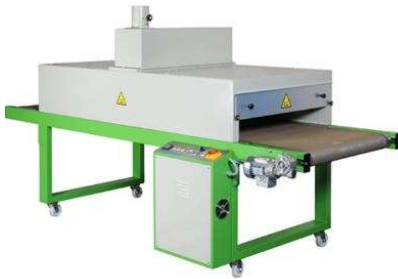
Figure 19: Drying and curing tunnel.
