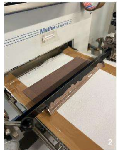
Figure 39: Application of a coating formulation. (1) Formulation poured on the substrate; (2) spreading.
