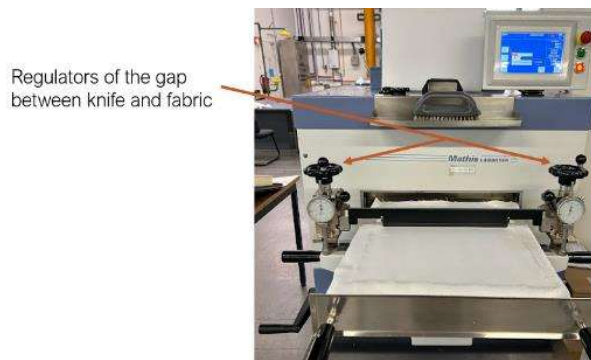
Figure 37: Fabric and knife prepared for coating, indicating the regulators of the knife's height.
