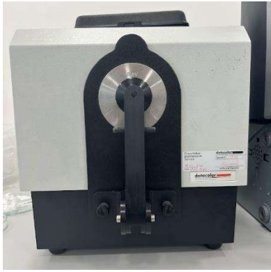
Figure 52: Datacolor® Spectraflash® SF450® - the machine that “reads” the samples.
