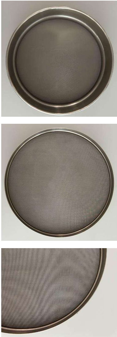
Figure 24: Different views of the Manual sieves used to achieve the 0.2mm particle size.
