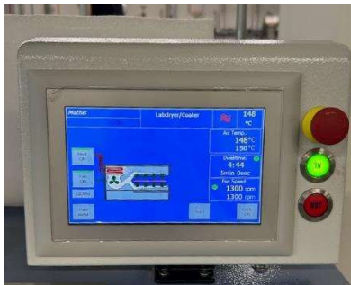
Figure 40: Display that shows the curing settings of a coating applications.
