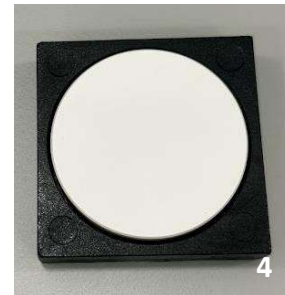
Figure 54: Patterns to calibrate the machine Datacolor® Spectraflash® SF450®. (1) and (2) different views of the black standard for the calibration; (3) and (4) different views of the white standard for the calibration
