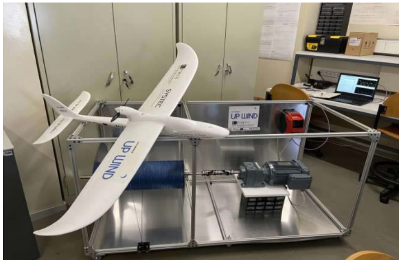
Figure 2.10: UPWIND Prototype with the Multiplex EasyStar II glider coupled to the ground-station [1].
