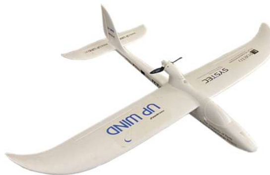
Figure 2.9: UPWIND Multiplex EasyStar II glider [1].
