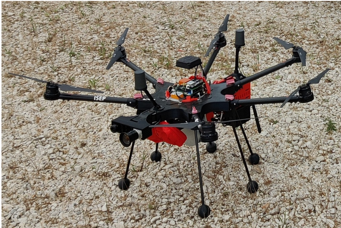
Figure 4.3: UAV Stork II equipped with first-aid rescue pack
