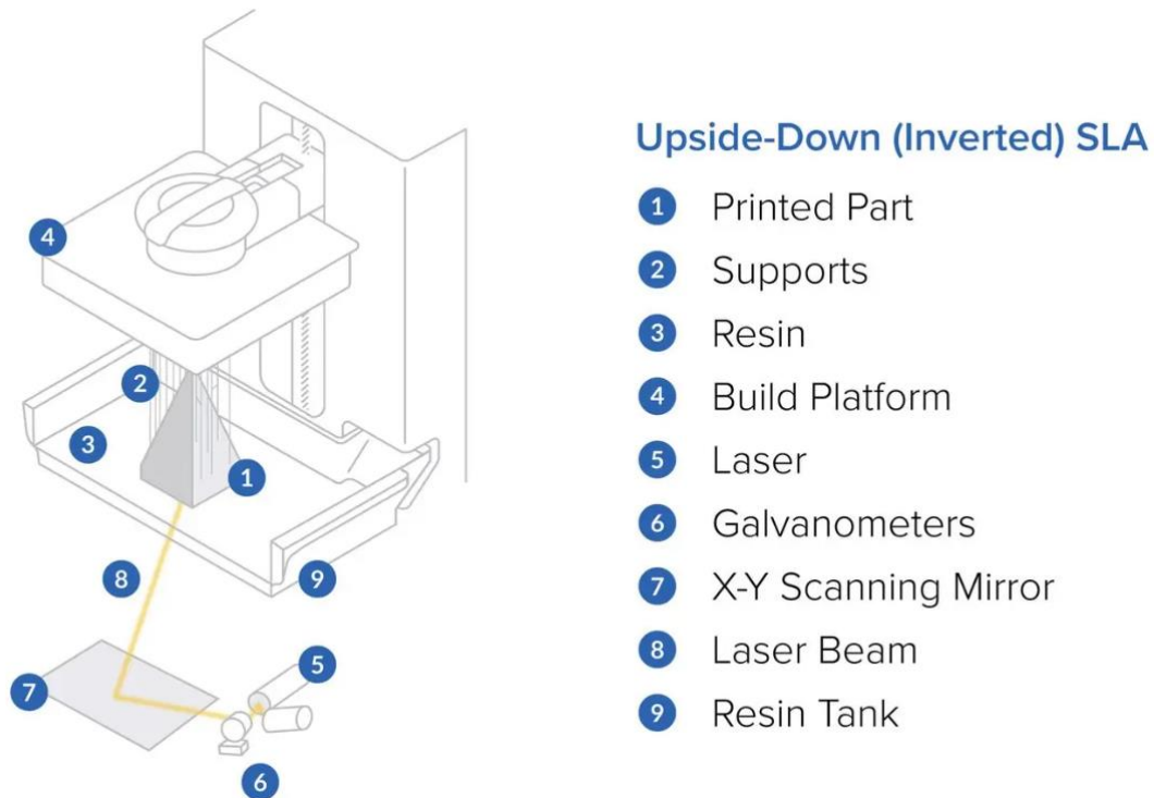
Figure 2.3. 3D printer scheme by Upside-Down SLA scheme; taken from: (FormLabs, 2023).
