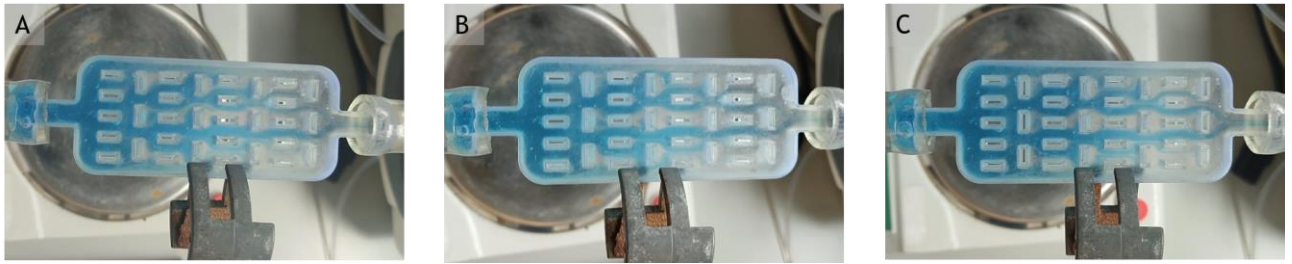
Figure 4.3. Frames of the video taken for the three tests when the first elements of fluid leave the domain: A) \omega = 30 rpm; B) \omega = 40 rpm; C) \omega = 50 rpm.
