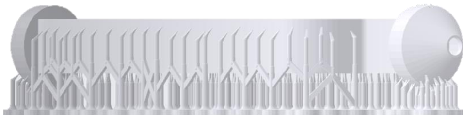
Figure 3.3. 3D Printing preview with the supports.
