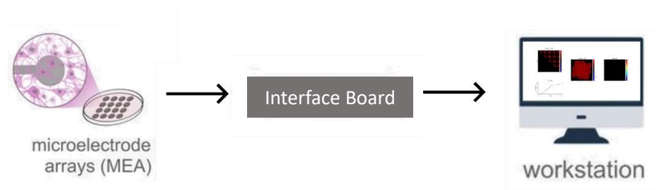
Figure IV-3. General pipeline developed for the analysis of real experimental data in “real-time”. Electrophysiological activity is recorded via microelectrode arrays, and transferred to a workstation in “real-time”. The data is processed by a connectivity inference algorithm, and the connectivity matrix and corresponding map is displayed for the user. Adapted from [17].
