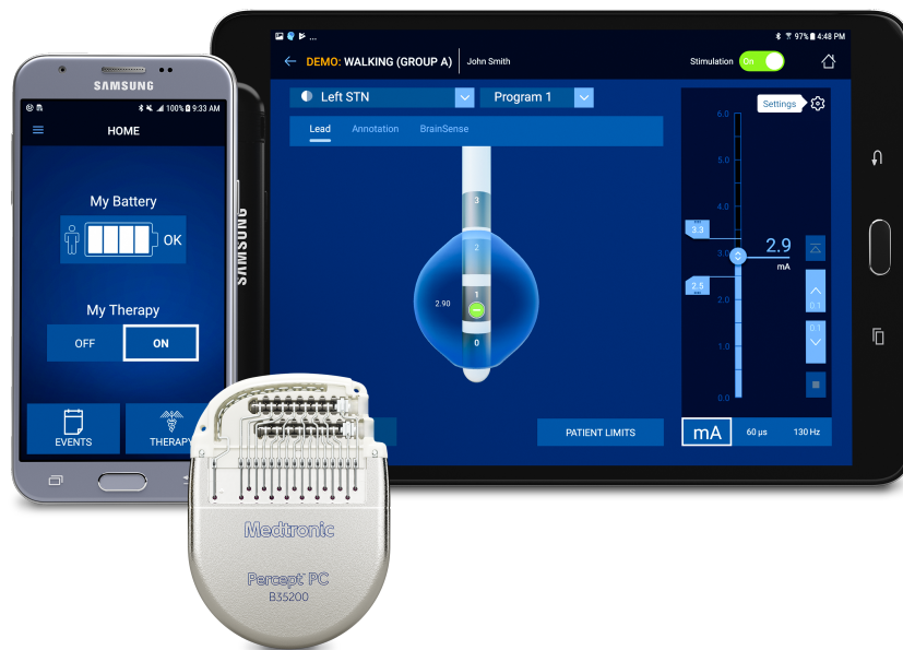
Figure 2.6: Percept™ PC Neurostimulator family: patient controller, dual-channel IPG, and clinician programming tablet (from left to right). ©2022 Medtronic. All rights reserved.
