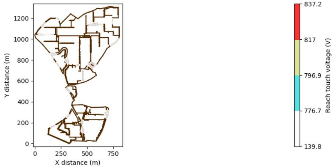
Figure 10.37 - Validation of the PV plant's touch voltages
