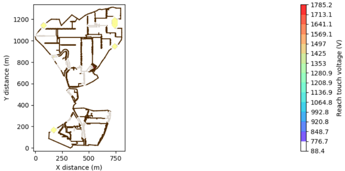
Figure 10.35 - Validation of the PV plant's touch voltages
