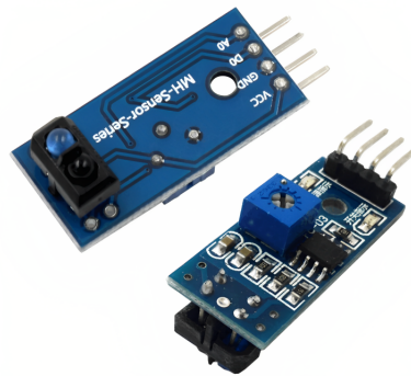
Figure 3.2: TCRT5000 module with analog pin [42]
