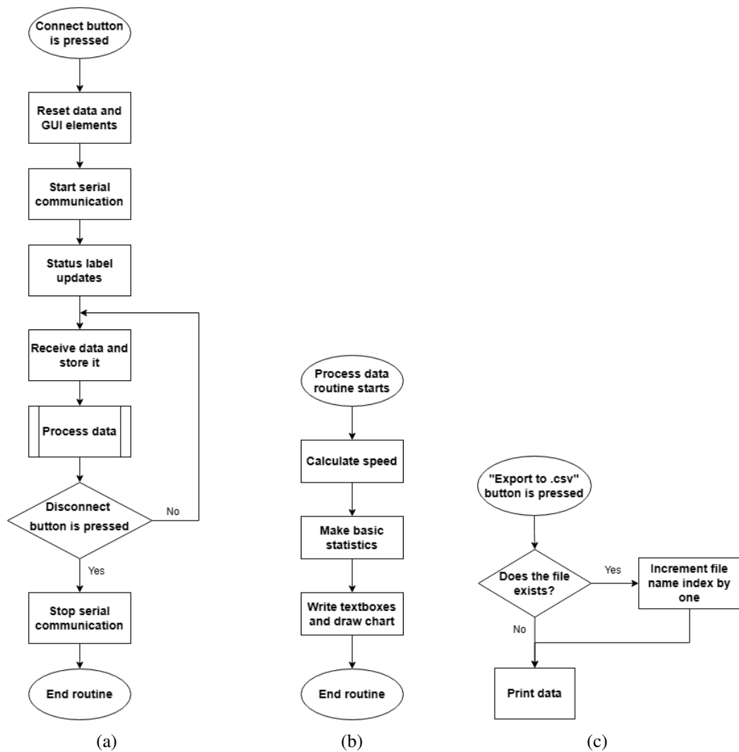
Figure 3.22: User's interface software code secondary flowcharts: a) Connection routine; b) Processing data routine; c) Exporting data to a .csv file routine.
