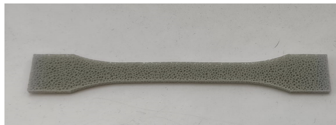
Figure 3.30: Traction specimen with 4000 points and 0.4 mm of thickness.
