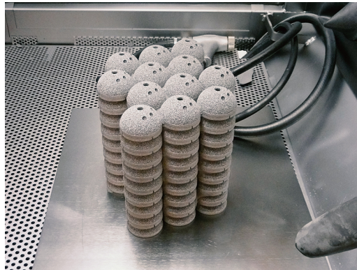
Figure 2.25: Production of metal components by SLM from GE Additive [76].
