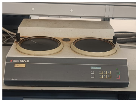
Figure 3.17: Struers RotoPol-21 machine used for the polishing and finishing of the optical microscope specimens.
