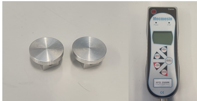
Figure 3.43: (Left) Compression fixtures. (Right) 2500 N load cell.
