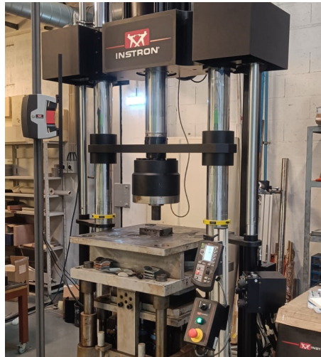
Figure 3.11: INSTRON 5900R test machine in INEGI, used for the compression tests.
