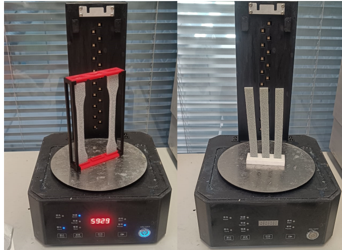
Figure 3.27: Post-cure procedure, with samples placed on different supports (in the back it is possible to see the UV lights used in the curing process). (Left) Traction specimens. (Right) Flexural specimens.
