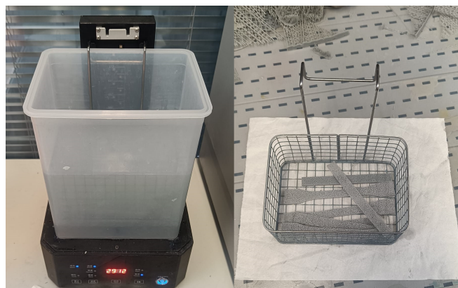
Figure 3.26: Cleaning procedure. To the right, the placement of samples in the cleaning basket. To the left, the immersion of the samples in the cleaning solution.
