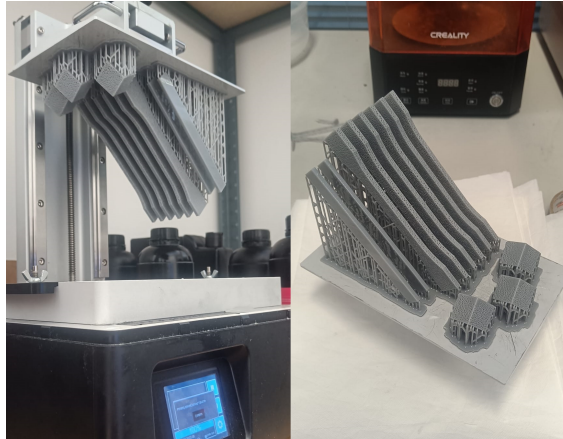
Figure 3.24: Example of a finished printing job, with traction, flexural, and compression specimens.
