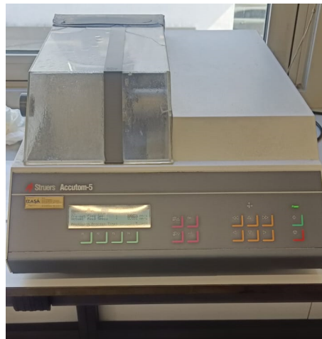
Figure 3.14: Struers Accutom-5 machine, used for cutting of the optical microscope samples.
