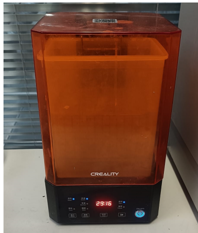
Figure 3.25: Creality UW-01 equipment, used for cleaning and curing procedures.
