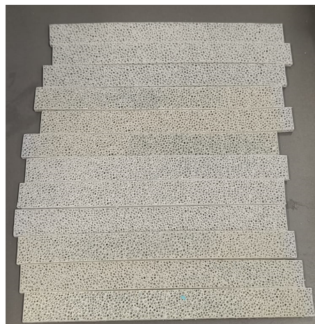
Figure 3.28: Resin flexural samples fully post-processed, ready to be tested.
