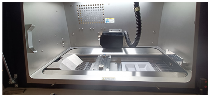
Figure 3.6: SLM machine printing chamber, with mounted recoater.
