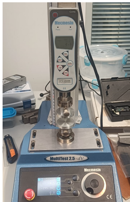
Figure 3.42: Mecmesin Multitest 2.5-dV testing equipment with the necessary compression test fixtures and load cell.
