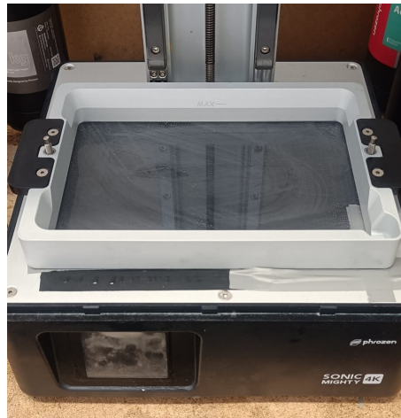
Figure 3.23: Phrozen Sonic Mighty 4K resin vat, displaying the maximum permitted resin level.
