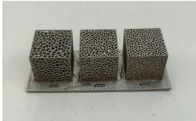
Figure 4.2: Set of 3 Voronoi structures with different number of points (2000, 4000, 6000).
