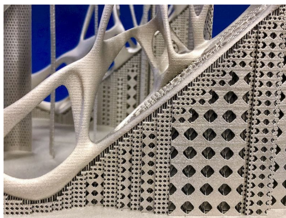
Figure 2.21: Example of SLM support structures [67].
