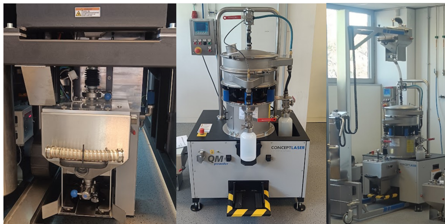
Figure 3.4: Metallic powder recycling process. (Left) Used powder container at the machine. (Middle) Vibrating screener. (Right) Recycling process in action, with used powder canister at the top of screener, and the recycled powder canister at the bottom of screener.
