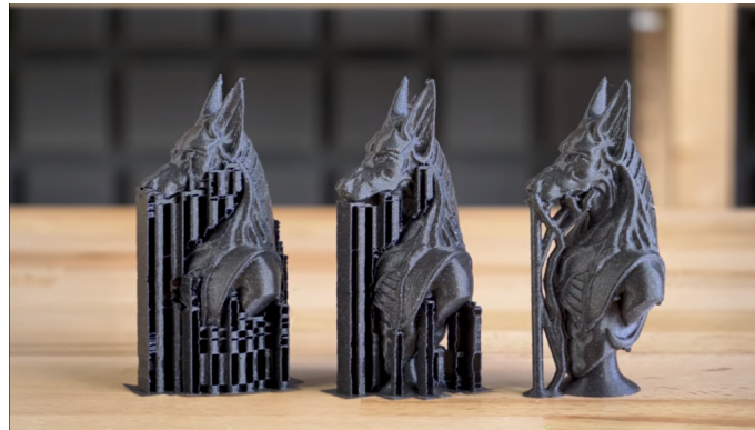
Figure 2.50: Example of the application of support structures, and subsequent optimization [97].
