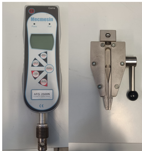
Figure 3.32: (Left) 2500 N load cell). (Right) Traction jaw fixture.
