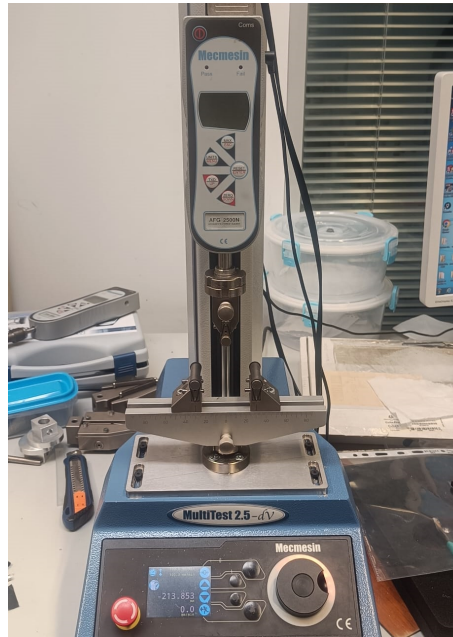
Figure 3.36: Mecmesin Multitest 2.5-dV testing equipment with the necessary flexural test fixtures and load cell.
