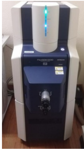
Figure 3.20: Hitachi FlexSEM 1000 scanning electron microscope.
