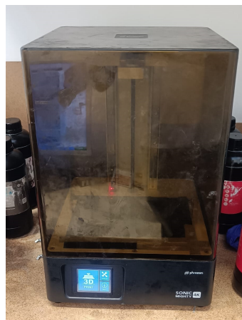
Figure 3.21: DLP machine Phrozen Sonic Mighty 4K.
