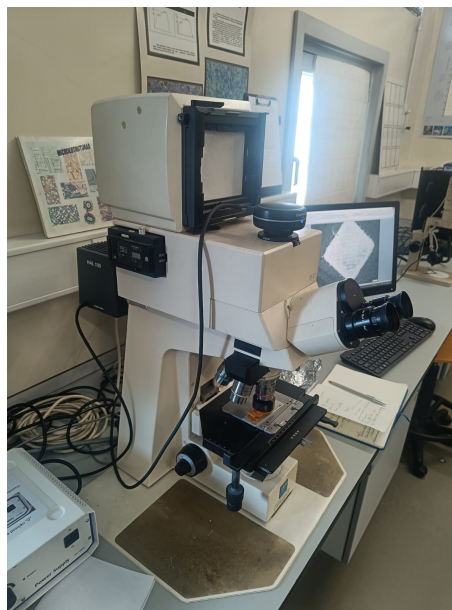
Figure 3.19: ZEISS Axiophot machine, used for the optical microscopic analysis
