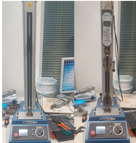
Figure 3.31: (Left) Mecmesin Multitest 2.5-dV testing equipment. (Right) Testing equipment with traction test fixtures and load cell.
