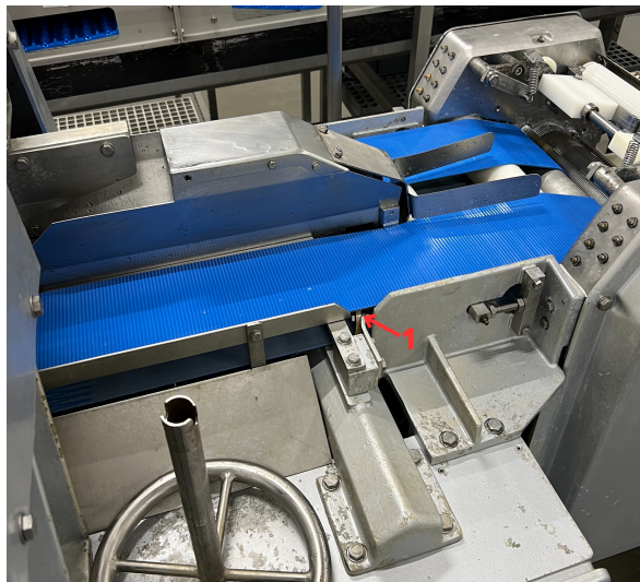
Figure 4.7: Area for implementing the fillet sensor
