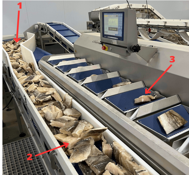
Figure 3.3: Production line – Initial part. 1- Dock, 2- Entry conveyor, 3- Weighing machine
