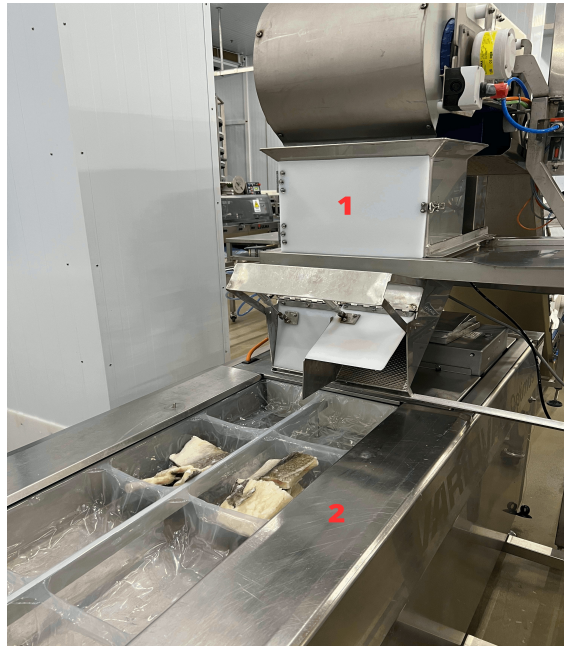
Figure 3.7: Packaging procedure. 1- Sorting machine, 2- Initial part of Thermoforming machine
