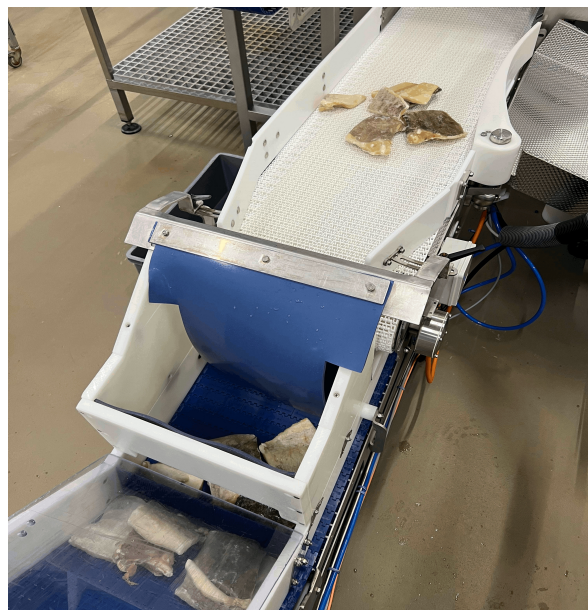
Figure 3.19: Product ready in supply conveyor and another dose already waiting
