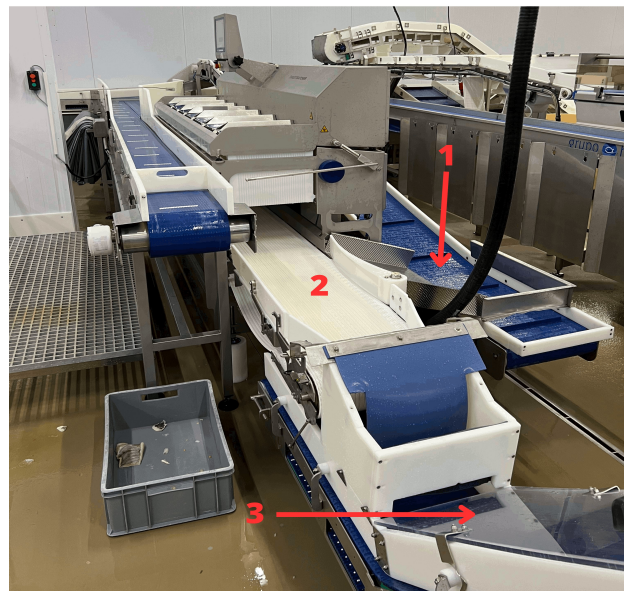
Figure 3.4: Production line – Part 2. 1- Return to Entry conveyor, 2- Dose conveyor, 3- Lift
