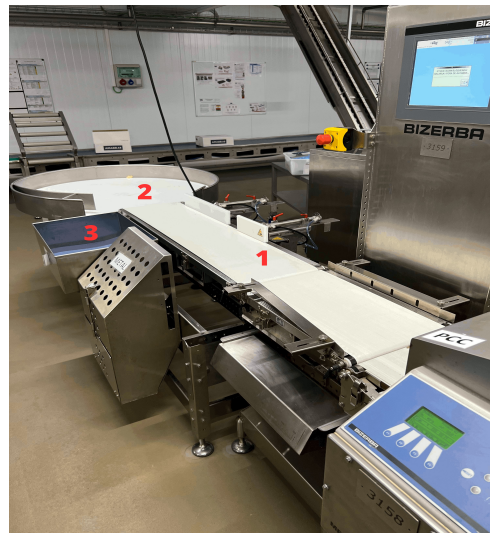
Figure 3.10: End of the production line. 1- Final conveyor, 2- Buffer, 3 - Trolley
