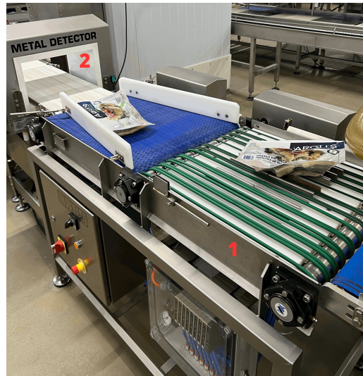
Figure 3.9: Exit conveyor of Thermoforming machine (1) and CCP (2)
