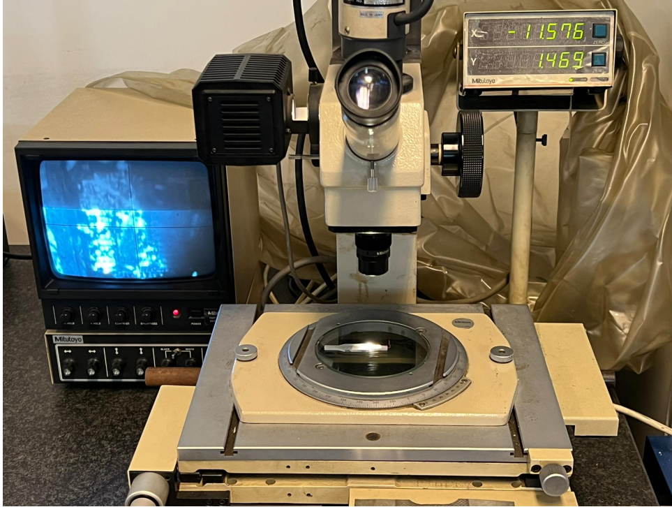
Figure 4.25: Flat specimen in Mitutoyo measuring microscope
