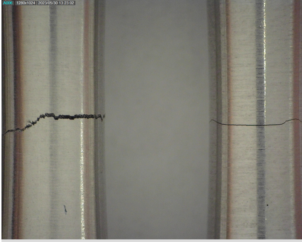
Figure 5.4: Surface and crack path comparison for polished and not polished smooth specimens
