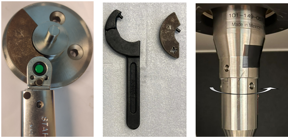
(a) Accessory to calibrate the torque wrench for 25 Nm (b) Tools to tighten the horn (c) Direction to tighten the horn
