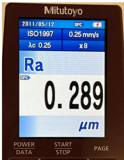
(a) Surface roughness of non polished specimen
