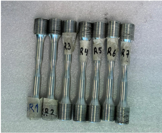
(a) M16 Smooth Specimens ( \phi 7 mm at gauge section)
