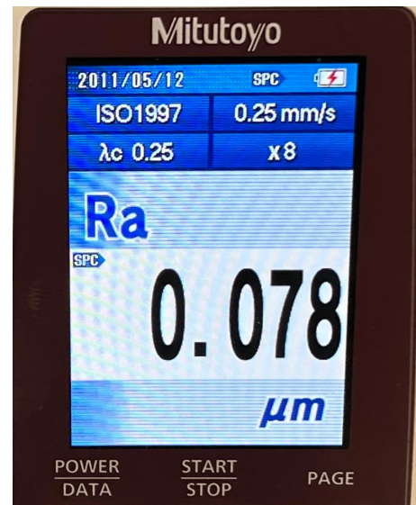
(b) Surface roughness of polished specimen
