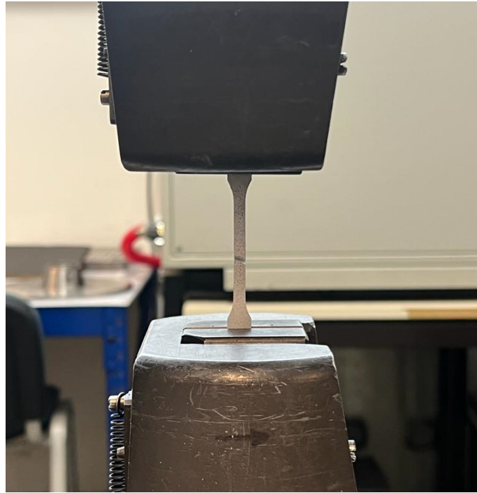
Figure 3.4: Tensile test on Al6082-T6 specimen
