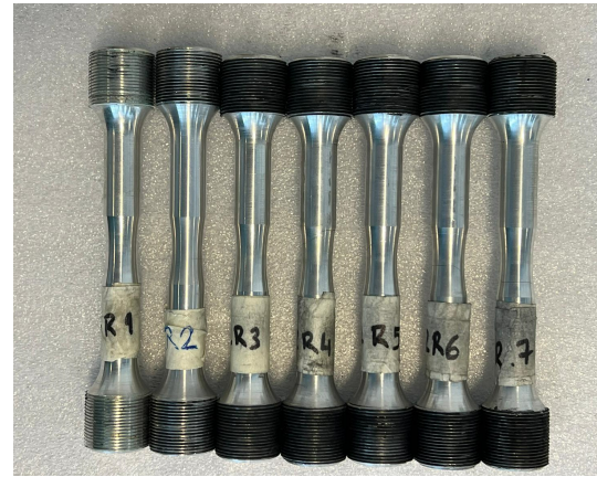
(b) M22 Smooth Specimens ( \phi 10 mm at gauge section)
